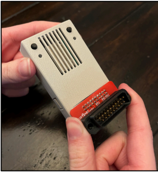
Remove the DB19 adapter by holding the PCB and gently rocking back and forth.
